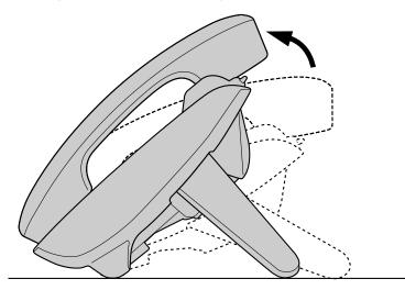
1. Tilt the stand in the direction indicated while pushing the PUSH mark with both hands as shown until it locks into the high position ().
