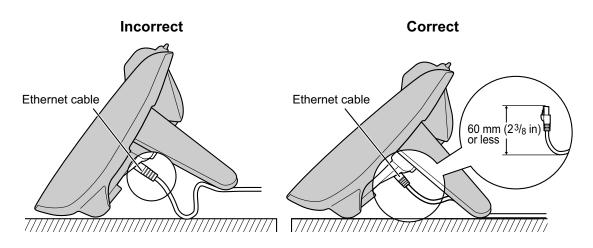
Use a straight CAT 5 (or higher) Ethernet cable (not included) that is 6.5 mm (<sup>1</sup>/<sub>4</sub> in) in diameter or less.
