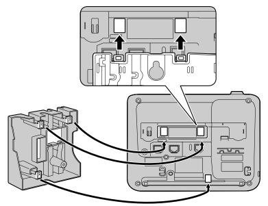
Fasten the wall mounting adaptor to the base with 1 screw. (Recommended torque: 0.4 N·m [4.08 kgf·cm/ 3.54 lbf·in] to 0.6 N·m [6.12 kgf·cm/5.31 lbf·in])
