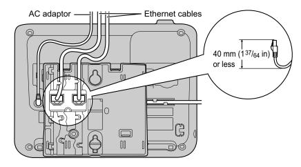
Drive 2 screws into the wall as shown in the illustration below, and mount the unit on the wall.
