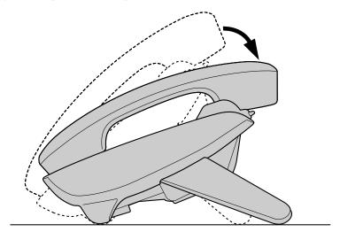
1. Tilt the stand in the direction indicated while pushing the PUSH mark with both hands as shown until it locks into the low position (**B**).
