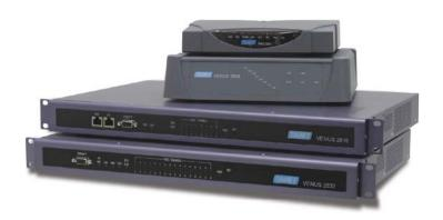
TAINET Communication System Corp. announces the VoIP Gateway solution is a line of purpose-built. The Venus Series VoIP Gateway is designed for empowering service providers to deliver Carrier-Class IP Centrex service over an Total-IP infrastructure NGN. Venus VoIP solutions support for multiple types of popular signaling protocols, MGCP, SIP and Megaco.
